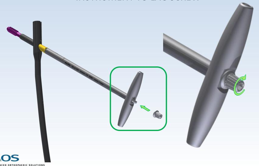
ROTATE T-HANDLE <u>CW</u> FOR ≈½ TURN, THEN BACK SCREW OUT BY ROTATING <u>CCW</u> AND PULLING LATERALLY UNTIL FULLY REMOVED.
